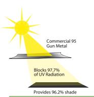
The %UVR block relates to the ability of the shadecloth to reflect or absorb Ultra Violet Radiation (UVR) within the 290nm to 400nm range of the spectrum. Heightened exposure to UVR has been shown to increase the rates of skin cancer. Therefore, the percentage of UVR block is an important factor when selecting shadecloth designed to protect people.
